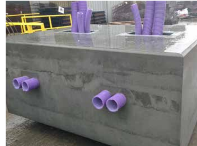
Precast communication bases with ducting cast in
