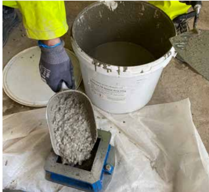
Making & Testing Concrete Cubes
