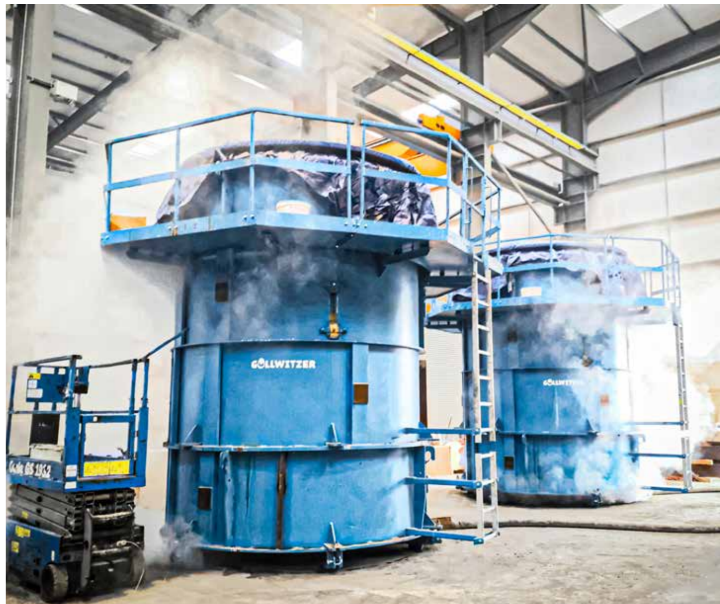
Wetcast jacking moulds during steam curing process
