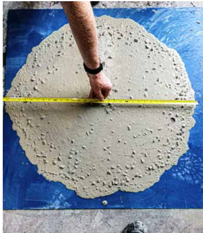
Flow test on concrete
