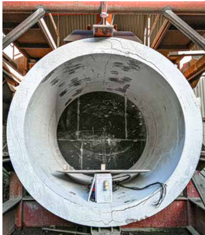
Crush Test on Jacking Pipe
